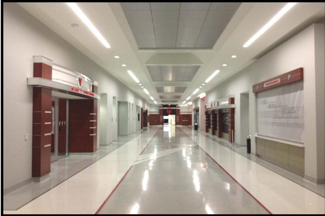
**Figure 2:** University of Tampa, Athletic Center. Duroplex installed over 5/8" Type X wallboard from 48" above floor, and over abuse resistant (AR) board from floor level to 48" above floor.
