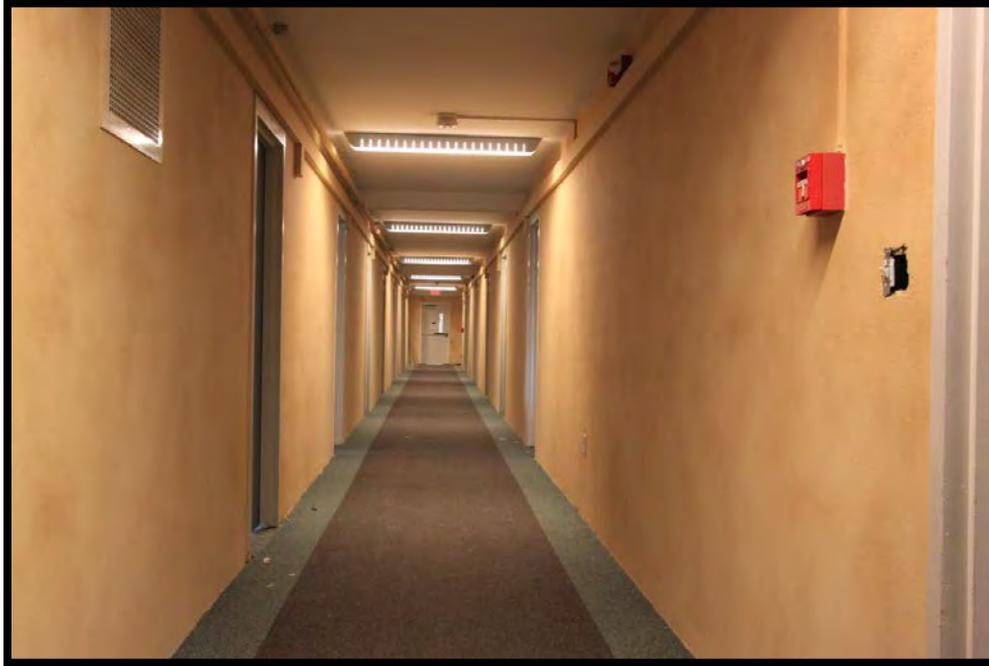
**Figure 6:** Shown above is the same corridor almost completed. The sequence of application was: PRIMER (X2), SKIMM, and Duroplex.
